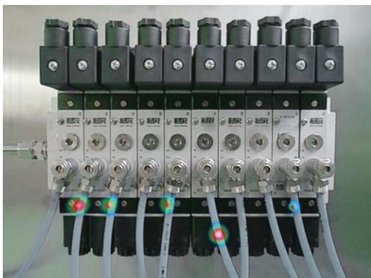
LeakCam 600 s 64 mikrofony (Power Beam Forming)
